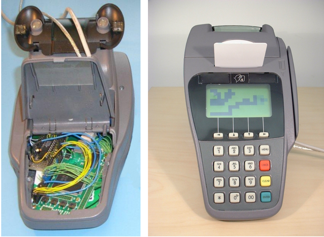
Figure 8: Modified Chip and PIN terminal, playing Tetris
